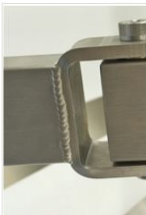
Cleaned weld- the burn marks are removed- the weld remains visible
