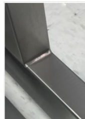
Ground Smooth- The weld is cleaned and grounded smooth- not invisible
