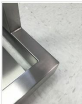
Polished weld Invisible weld
